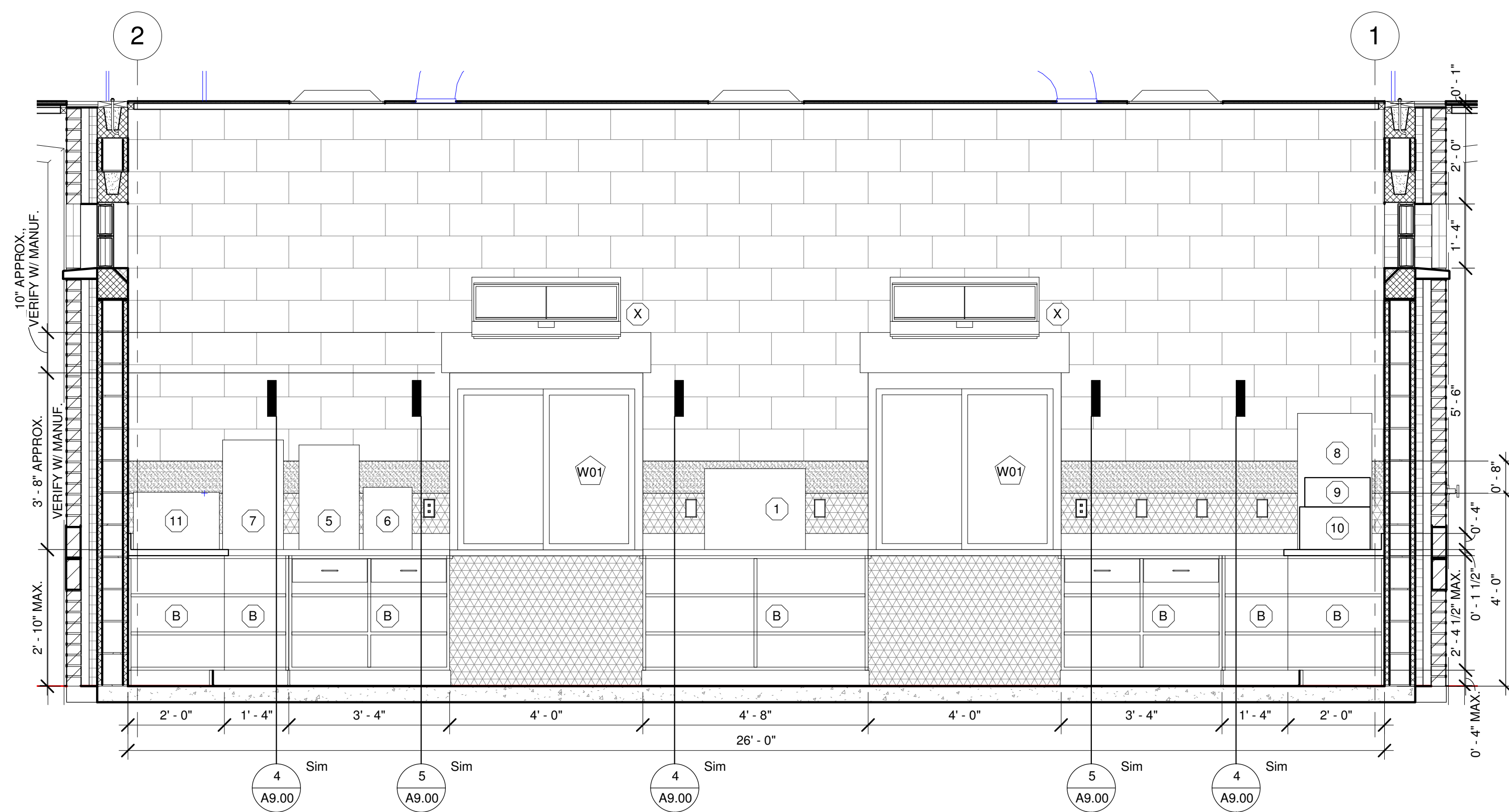
1 BLDG. A - CASEWORK ELEVATION 1 A9.01 1/2" = 1'-0"
